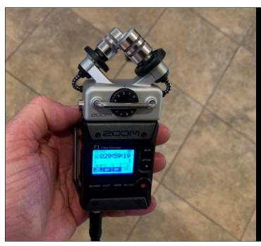
The two mics mounted on top of the Zoom F1 are for separately recording ambiance noise:
